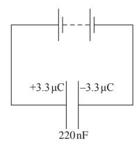
(a) Calculate the e.m.f. of the battery and the energy stored in the charged capacitor.
