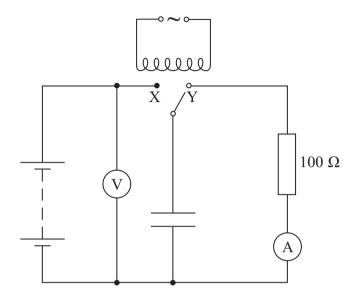
The switch flicks between contacts, X and Y, so that the capacitor charges and discharges f times per second.
